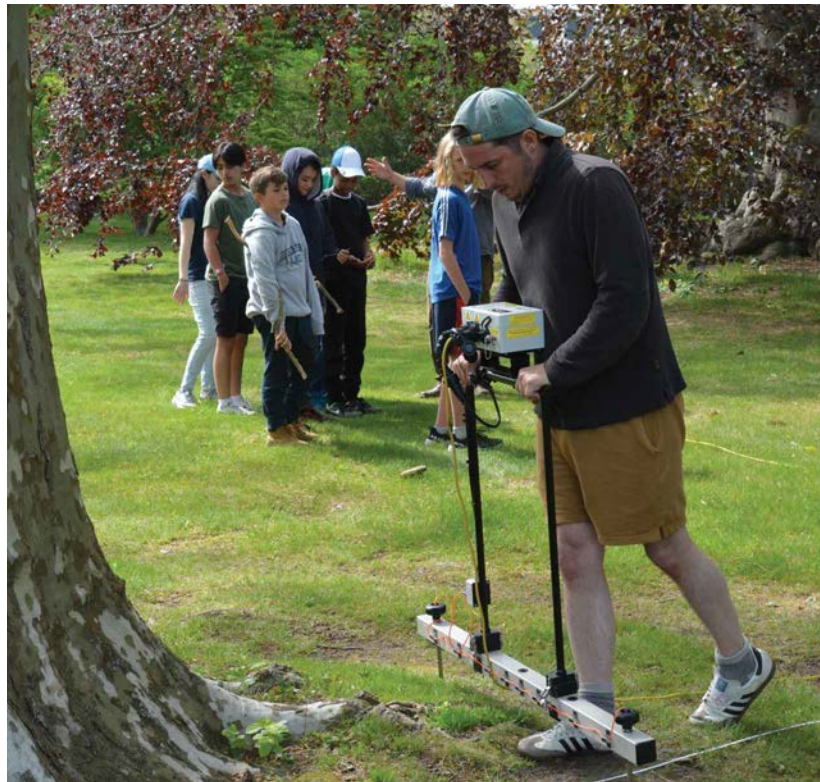
Professor & students from Dartmouth College & students from & FabNewport conduct ground-penetrating radar surveys at Kingscote.
